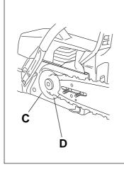
2 The front hand guard is not designed solely to activate the chain brake. Another important safety feature is that it prevents the chain from hitting your left hand if you lose your grip on the front handle.
